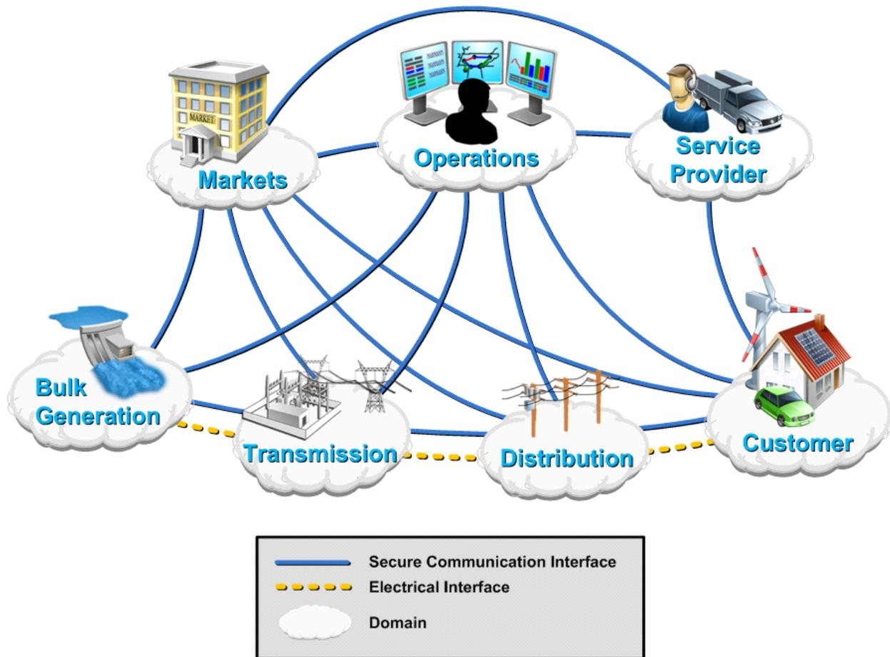
Figure 3 – Smart Grid Conceptual Model – Top Level
