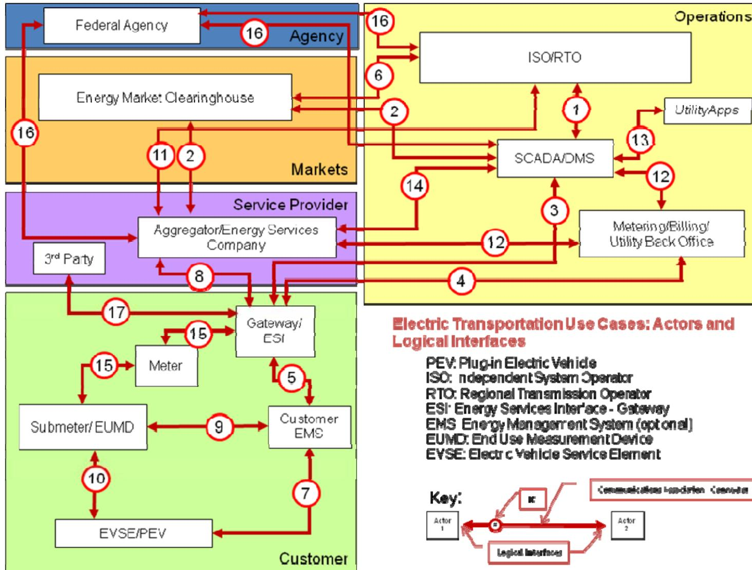
Figure 18 – Electric Transportation Applications Summary Communications Diagram
